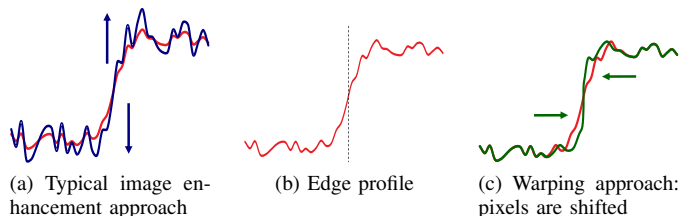
Fig. 1: The idea of edge sharpening by grid warping.
