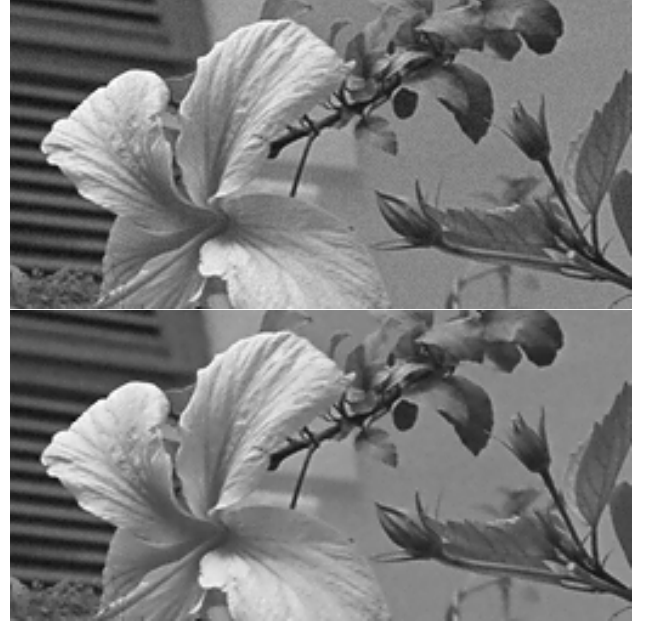
Figure 5. Denoising by the proposed method. TID image I07, noise \sigma = 4 .
