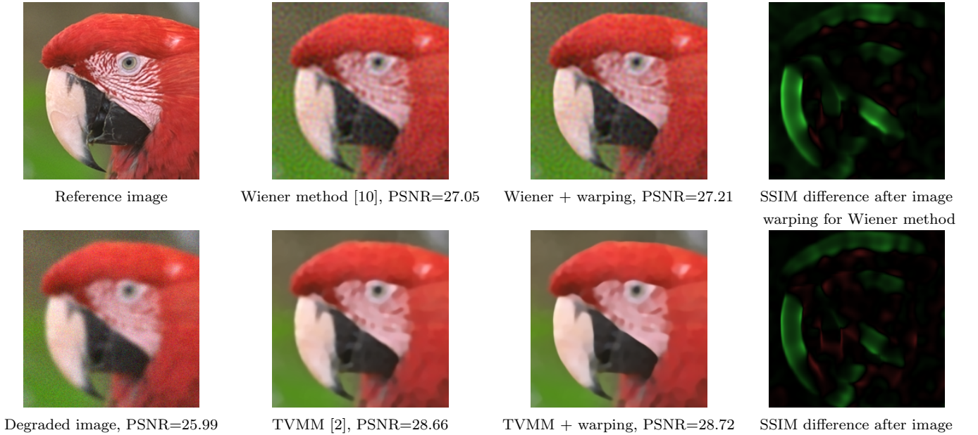
Figure 3: Poisson warping algorithm example. Green areas show improvement of SSIM, red — degradation.
