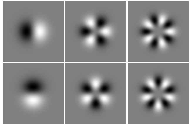
Figure 1: The real parts of g_0^1 , g_0^3 and g_0^5 (upper row) and the imaginary parts of g_0^1 , g_0^3 and g_0^5 (lower row).
