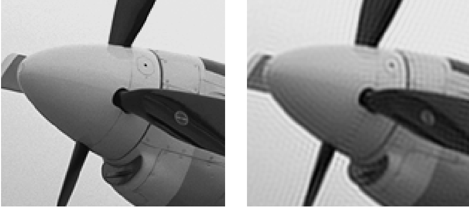
Fig. 1. Example of the ringing effect: reference image (left) and image with ringing effect (right).
