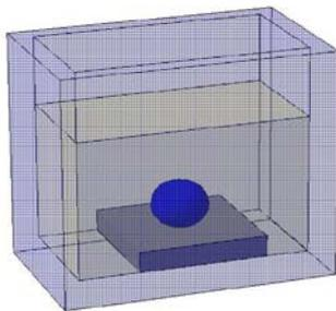
Fig. 6. Water drop on PTFE substrate immersed in octane.
