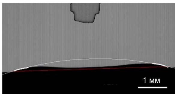
Fig. 9. Contact angle measurement of the spreading drop of molten NaCl
