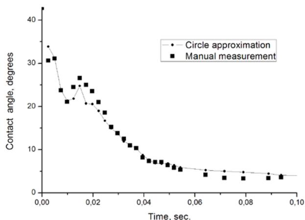
Fig. 10. Time dependence of contact angle for NaCl drop spreading over hydroxyapatite substrate.
