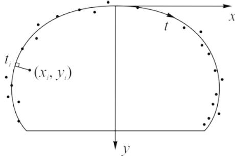
Fig. 1. Theoretical drop shape (solid line) and experimental points (dots).
