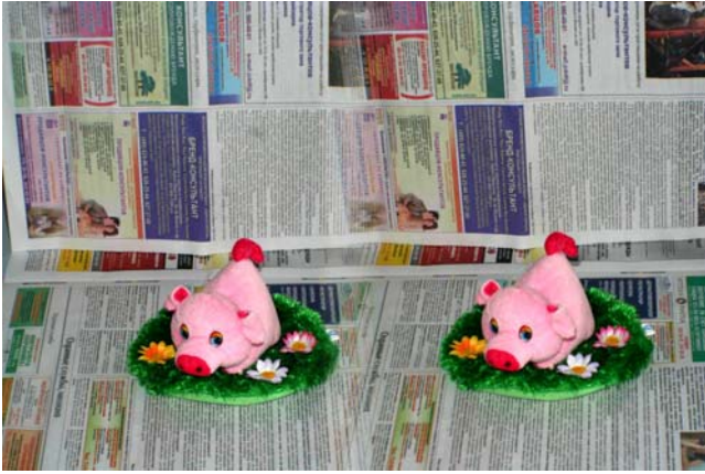
Figure 1. Example of stereo pair of images used to find 3D cloud of points.
